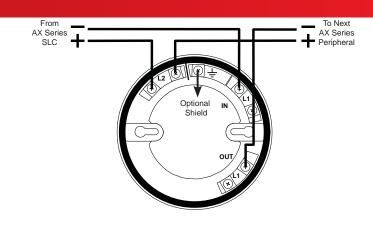
Intelligent Isolating Detector Base Wiring, 45681-321ADV
