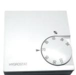
Measuring element: Contact type: Switching capacity: Settings: Housing: Dimensions (WxHxD): Connections: Protection rating: Bimetal switch 1 Change-over switch 230 V AC / 5 A 35 – 10% humidity Surface mounting, plastic, white 74,5 x 74,5 x 25 mm Screw terminal 1,5 mm<sup>2</sup> (rigid wire) IP30
